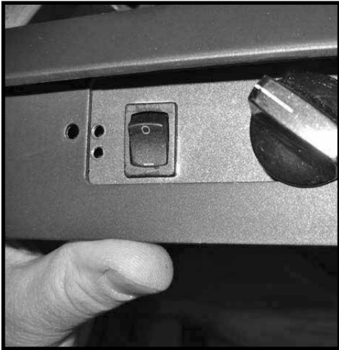
Figure 25: Reinstalling the Speed control assy.
