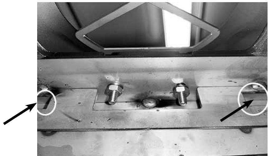
Figure 10: Front mounting slots for Flue Gas Agitator.
