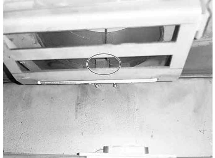
Figure 6: Remove Flue Gas Agitator
